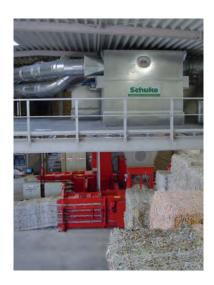
Schuko separators separate the suctioned material from the air current and feed it to press containers or bale presses (see photos at left and above). The dust loaded air current continues its path to the filter, where the dust is separated and the filtered air is re-circulated to the production halls. This saves energy and ensures a pleasant atmosphere in the working areas.
