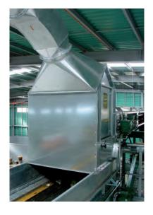
A large control window enables full control of the adjustment of the air separator for optimum sorting results.
