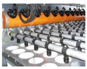
Stationary compressed air regeneration. The maintenancefriendly plug-system with an optimized compressed air tank and redesigned outlets prolongs the lifetime of the filter hoses.
