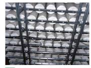
2 Increased filter surface allows malfunction-free performance of the extraction system. Raising the filter surface by 21% per element enables an even more effective strain of the filter material and prolongs the lifetime of the filter hoses
